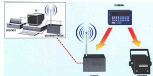
Fork lift truck scales including our electronic weighing units may be delivered works-calibrated and may be suburb installed by the customer.
