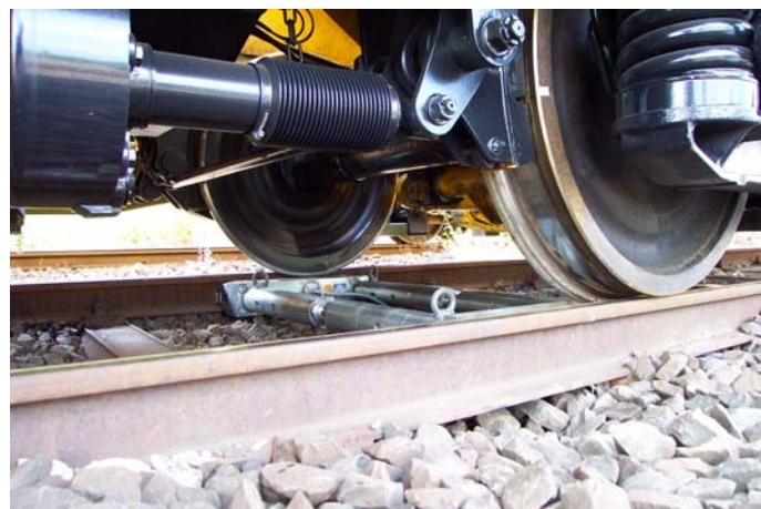
MEW 2008 in heavy-duty version up to a maximum wheel load of 15 t (with 2 beams)
