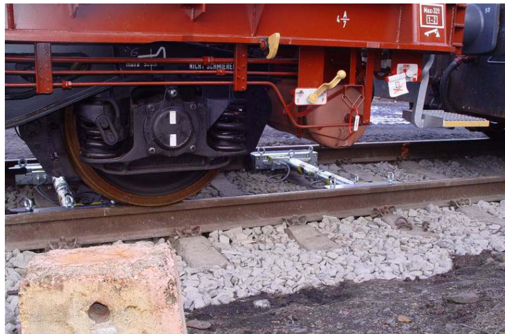
MEW 2008 standard version with 12.5 t wheel load in use
