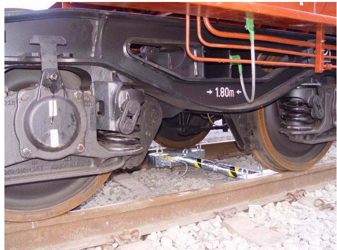
MEW 2008 in standard version up to a maximum wheel load of 12.5 t (with 1 beam)
