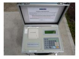
Case Dimensions: 430 x 310 x 150mm (H) Weight: 6.5Kg Powered by 240v plus a self contained re-chargeable battery. Battery life approx 1 week with overnight recharge via 240vVadaptor.
