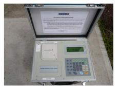
Case Dimensions: 430 x 310 x 150mm (H) Weight: 6.5Kg Powered by 240v plus a self contained re-chargeable battery. Battery life approx 1 week with overnight recharge via 240V adaptor.
